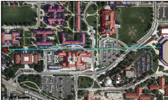
EDX's ray-tracing models make use of exact descriptions of the buildings and other features of the environment where your wireless network will be deployed. You can independently specify the conductivity, permittivity, transmission loss, and wall roughness as a function frequency for all the building and wall features describing your environment. The model calculation results include:
